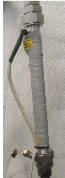
Figure 5: New humidifier assembly with attached heater module.
